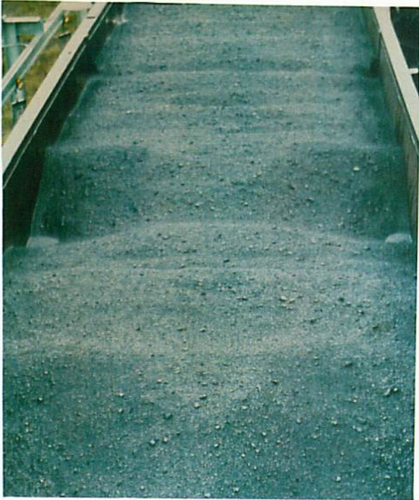
《 PLATE NO.3: UNTREATED CAR SHOWING POOLS OF WATER AND COARSE COAL
