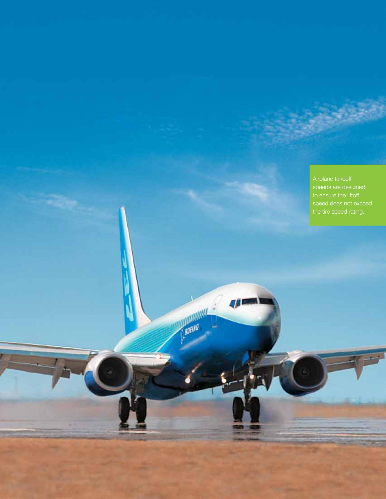
Airplane takeoff speeds are designed to ensure the liftoff speed does not exceed the tire speed rating.
