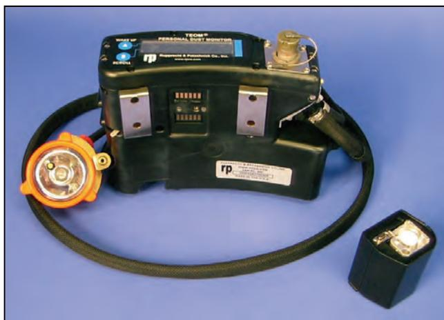
Figure 2-3.—PDM with TEOM removed (*shown on right*).
