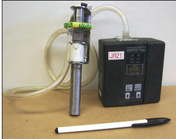
Figure 2-1.—Gravimetric sampling pump, cyclone, and filter cassette.
